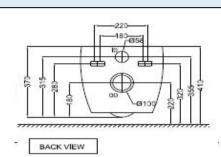
ALL DIMENSIONS ARE IN MM (TOLERANCE ± 5 MM)
